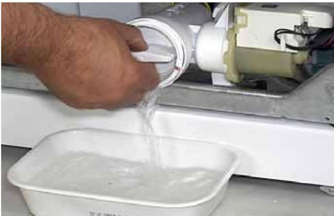
5. **TECH TIP:** If water is seen in the washer, there may be too much to catch all at one time. Loosen the filter, but do not remove it. Secure the filter when water reaches a depth that is easy to carry. Dump the collected water and return the pan to catch the remaining water.
