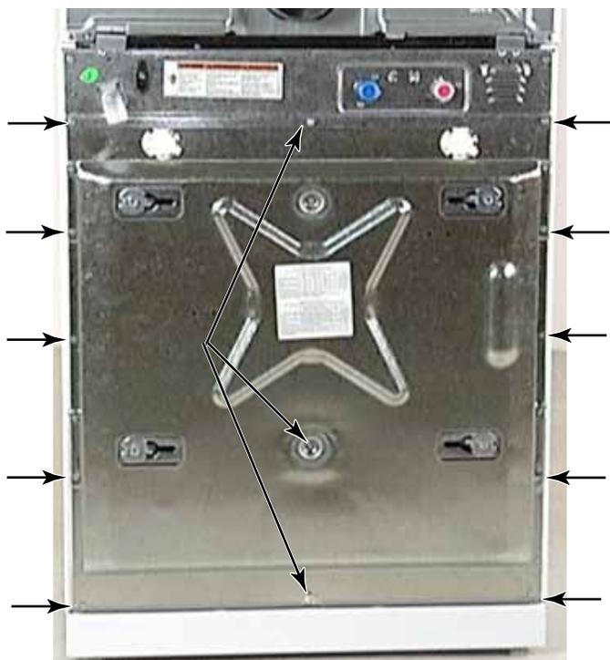
4. Pull the bottom edge out and slide the panel down from behind the lip at the top edge to remove the panel.
