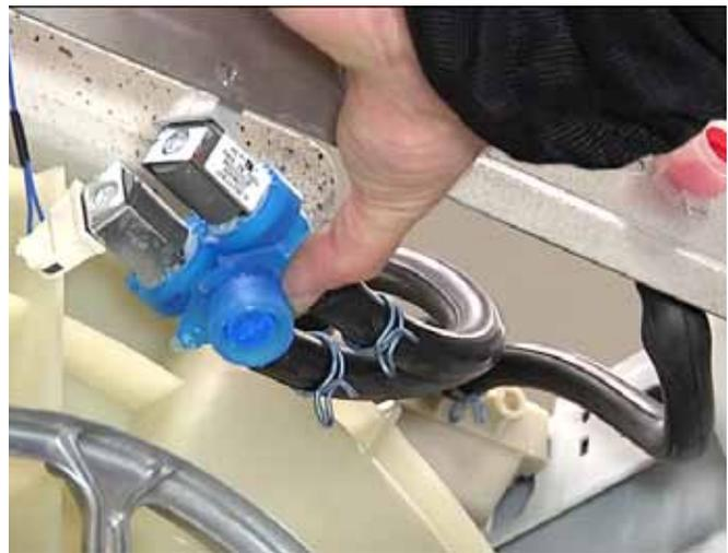
9. Lift the locking tab and disconnect the rast connector from each of the two cold water inlet valves.
