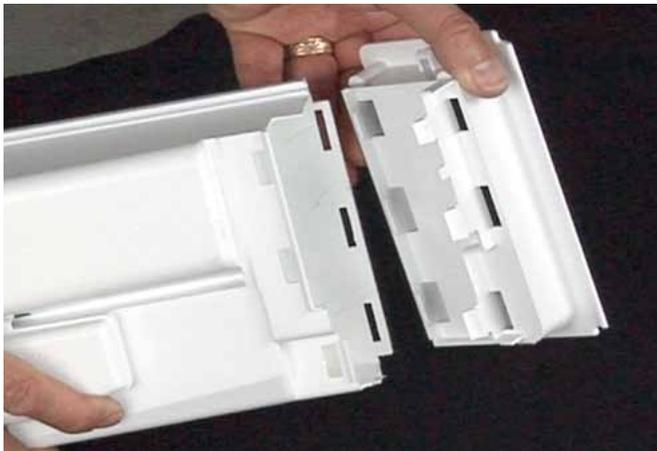
12. There is a bottom cover under the bleach and fabric dispenser cups. This cover should be removed and the siphon holes cleaned to maintain good elimination of chemicals during the cycle.
