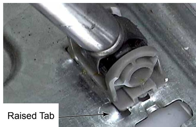
**TECH TIP:** When removing the tub, the air gap dampers simply separate when the tub assembly is pulled up out of the washer.
