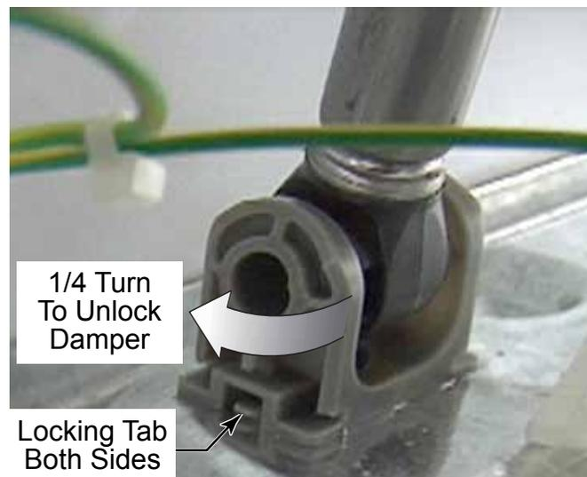
8. To separate the two halves of an air gap damper, Disconnect either the bottom or the top of the air gap damper from the washer. Slide the two halves of the air gap damper apart to separate them.
