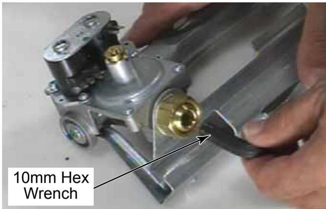
3. Turn the fitting counterclockwise to unscrew it from the gas valve.
