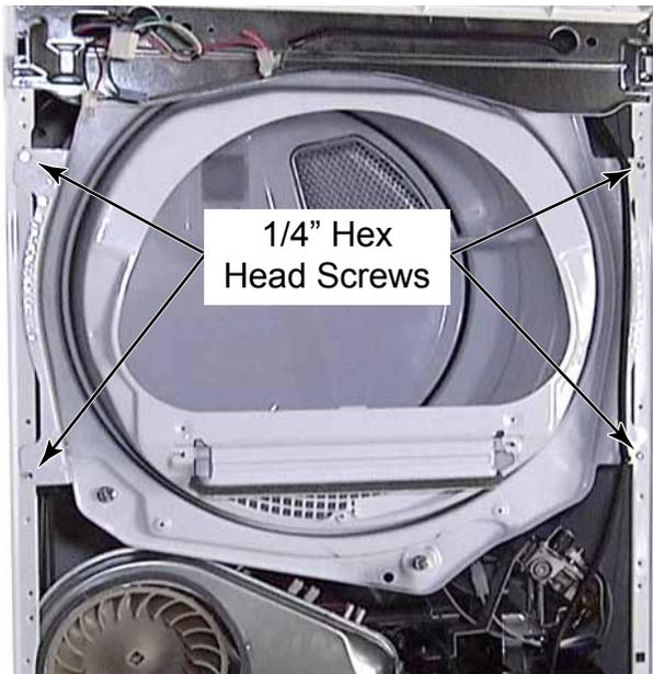
4. Lift the right side of the front bulkhead so the top screw can pass through the snowman hole. Pull the bulkhead away from the dryer enough to reach the Christmas tree clips inside.
