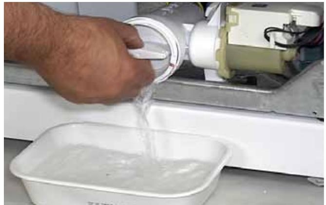
14. Disconnect the drain hose from the back of the pump filter. Move the clamp down the hose. Pull the drain hose off the back of the pump filter.
