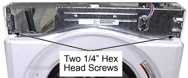
10. Remove the front panel from the washer.
