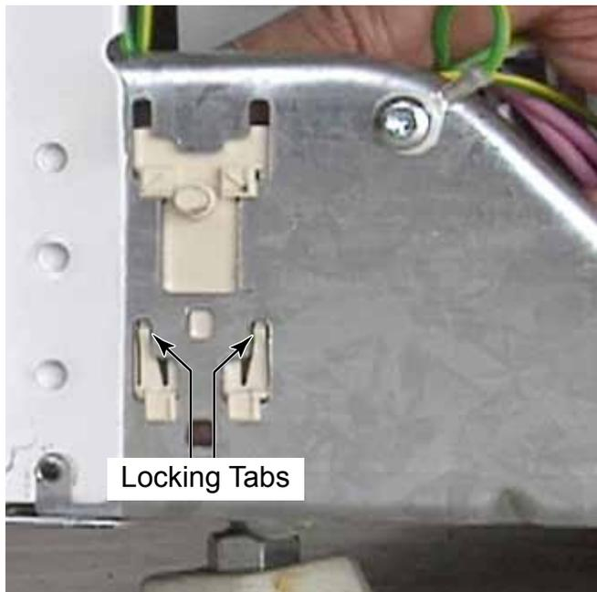
4. Slide the switch up and pull it out of the slots to remove it.
