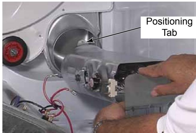
5. Remove assembly from the dryer.
