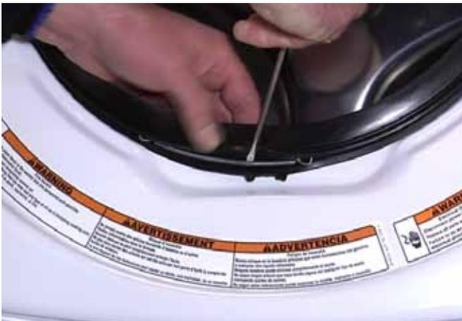
5. Peel the bellow off the edge of the front panel and push it into the cabinet opening in the upper left corner.
