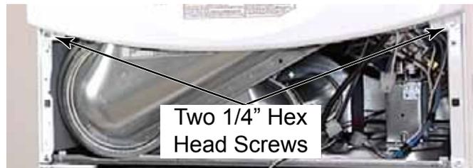
8. Remove two 1/4" hex head screws securing the top of the front panel to the dryer. These screws were hidden behind the dryer console panel. Make sure to support the front panel when removing the screws so it does not fall.
