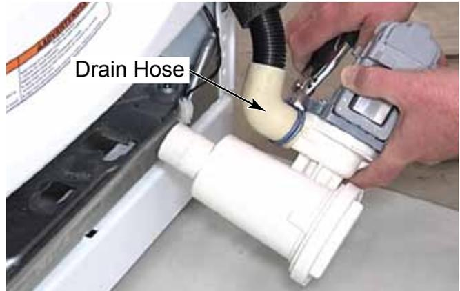
17. The two screws securing the rubber mounting piece to the bottom of the pump support do not need to be removed to remove the pump assembly.
