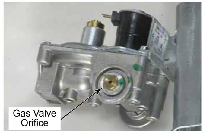
**TECH TIP:** When replacing a gas valve assembly it is always prudent to remove the orifice from the original gas valve and install it on the new valve. This helps avoid having the wrong size orifice on the dryer after a gas valve replacement.
