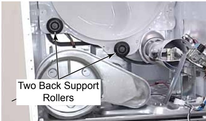
3. Slide support roller off the shaft.
