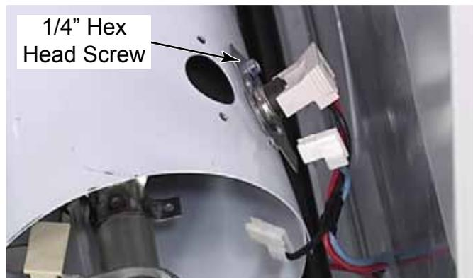
**TECH TIP:** If the burner thermal limit is being replaced, the burner high limit should be replaced as well, since the burner high limit should have shut the heat off before the dryer reached the temperature at which the burner thermal limit would trip.
