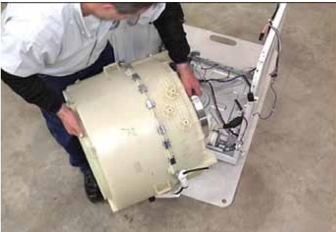
23. After the tub assembly is properly hanging from the upper support springs, align and insert the air gap damper tubes mounted on the base into the damper tops mounted on the tub before reinstalling the weights and motor on the tub assembly.
