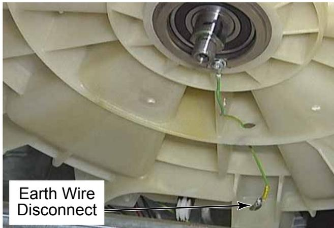
16. Remove the wire retainers by pressing the Christmas tree clips out of the holes in the bottom of the outer tub.
