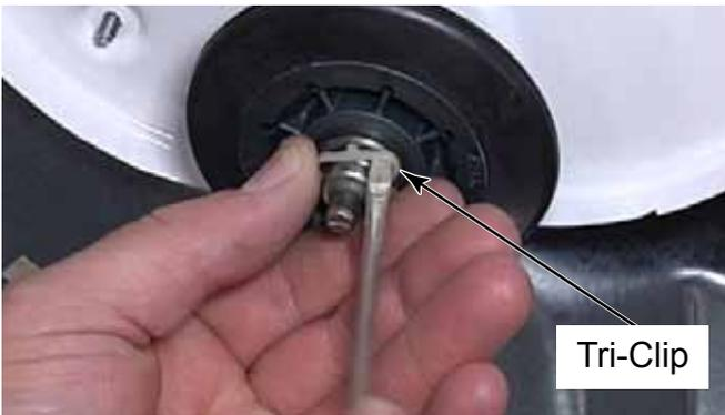
**NOTE:** When replacing a roller, always replace both tri-clips to make sure the roller will stay in position while running.
