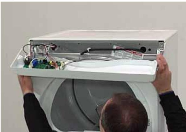
3. Lay the console cover forward to access the dryer control board.
