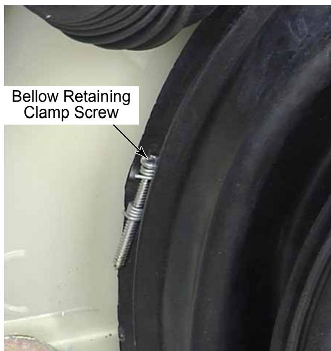
4. Remove the bellow retaining clamp from
