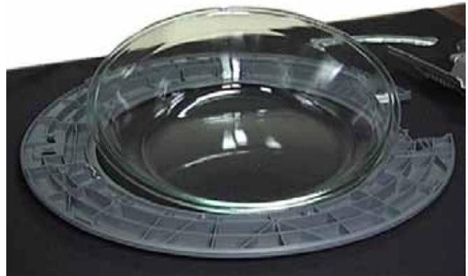
9. To remove the bowl, remove the hinge and remove three T-20 screws from each of the two brackets secured to the inner door panel. These screws also have threads for plastic but are shorter than the screws securing the door halves together.
