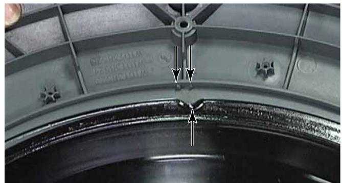
10. Support the inner door trim to avoid having it drop when removing the bowl brackets.
