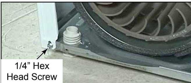
4. Remove two 1/4" hex head screws from lower back edge of side panel, one from the corner into the base and one above that into back bulkhead.
