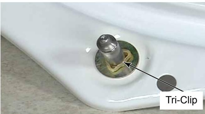
**NOTE:** DO NOT lubricate this wheel or shaft. Lubrication attracts lint and dust which will cause premature wear of the support bearing. Clean shaft with fine steel wool to eliminate squeaks, or replace worn rollers.
