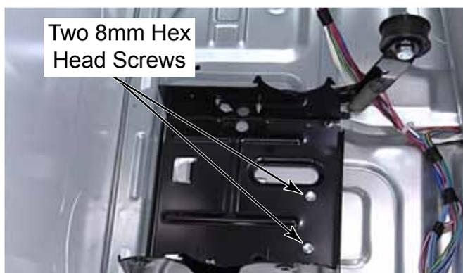
3. Lift the bracket and pull to the right to remove the two tabs that pass through the dryer base.
