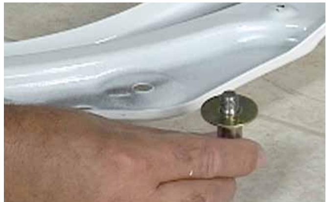
**NOTE:** To support the roller shaft while trying to remove the 14mm (9/16") nut a locking pliers needs to be used to hold the tip on the front of the roller shaft.
