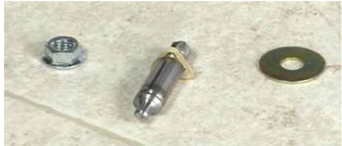
5. The washer is installed on the roller side of the shaft.
