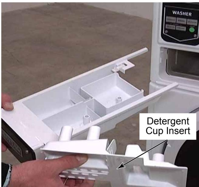
5. To remove the detergent flapper, place a flat blade screwdriver in the slot between the hinges at the top of the flapper and twist both ways to release the flapper.
