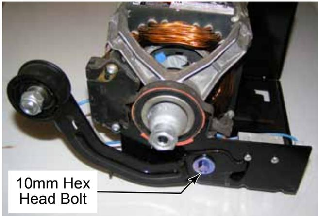
3. The mounting bolt has a shoulder and a permanent washer.
