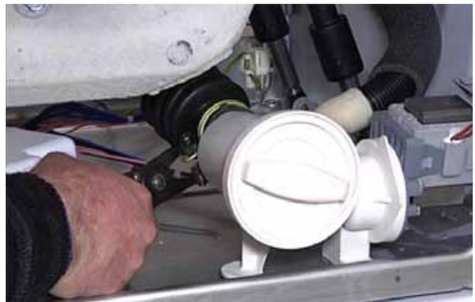
15. Disconnect the earth wire to the hub at the spade connection about 30cm (12") from the hub. Follow the earth wire down from the hub to the connector to locate the disconnecting point.
