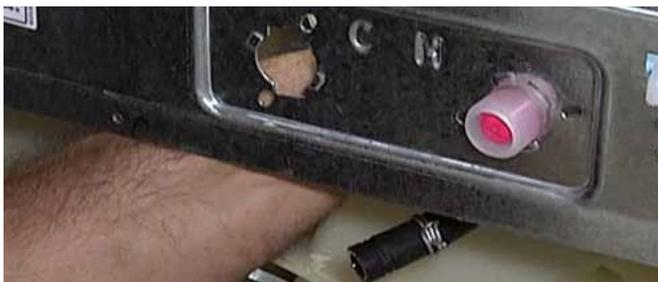
7. Pull the valve out of the hole in the panel and lower it to gain access to the hose clamps and Rast connectors.
