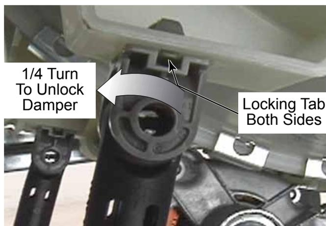
7. The damper is attached to the base in the same way, with 2 locking tabs.
