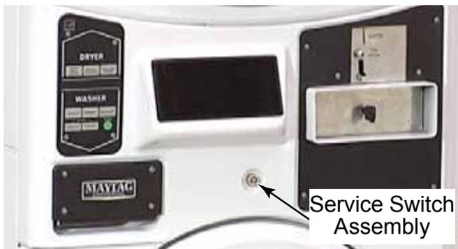
2. From inside the control panel, press the locking tab and disconnect the wire harness to the service switch from the control board.
