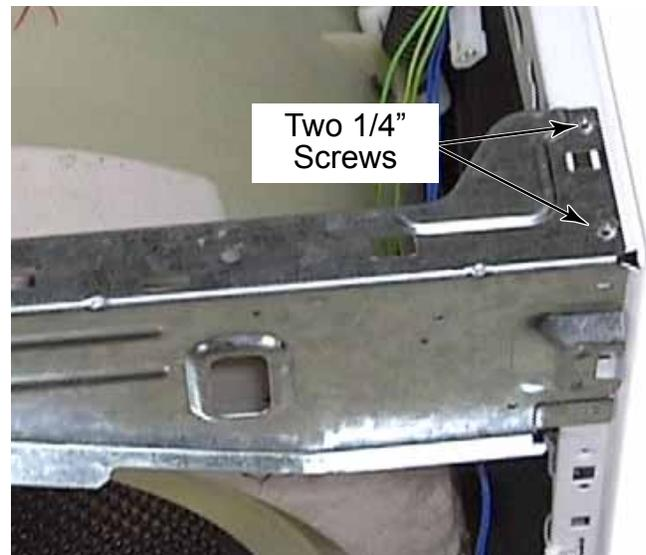
8. Lift the bracket and remove it from the washer.
