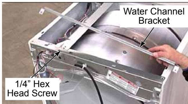
9. Pull the console bracket forward and lift the brackets up and place them on top of dryer.
