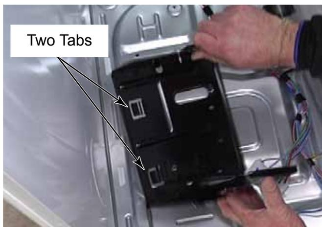
4. Remove the bracket from the dryer.
