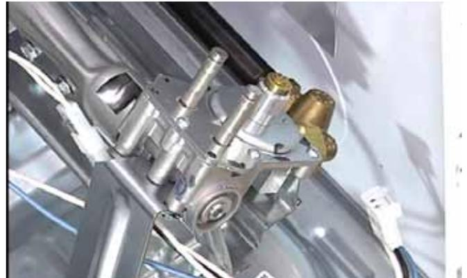
7. There is a locating pin on the top of each coil that fits into a hole in the bracket for proper orientation of each coil.
