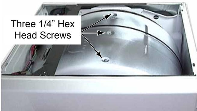
**NOTE:** These screws have multiple thread depths that grab plastic securely to help avoid screws becoming loose from vibration.
