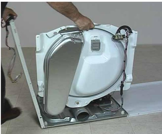
4. Use a pair of pliers to squeeze two Christmas tree clips to release wire ties holding wiring harness to back bulkhead.
