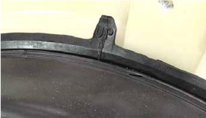
8. Wrap the top of the bellow over the outside edge of the outer tub, and at the same time press the inside lip of the bellow between the outer tub and the spin basket.
