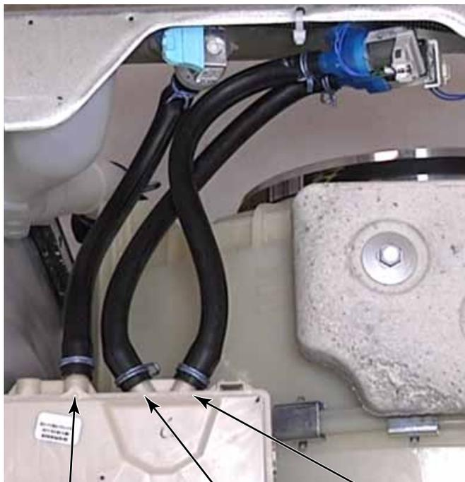
Hot Water Valve 1      Lower Cold Valve 3      Upper Cold Valve 2
