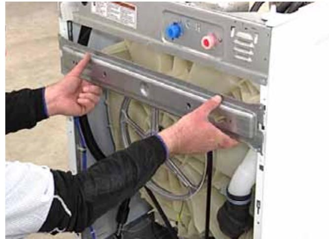
**NOTE:** With the dryer mounted to the top of the washer it is not recommended that a washer cross brace be removed. When the dryer is removed from the stack, if one or both braces are removed for any purpose, do not move or lean on the washer because the side panels will be damaged.
