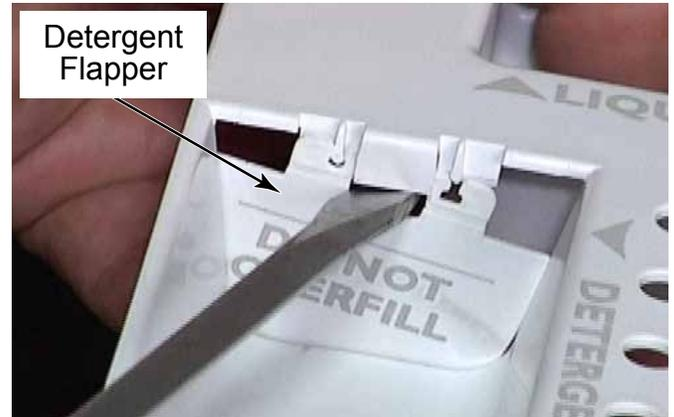
6. The locking tab can be removed by unclipping it from slots in the top left back corner of the chemical dispenser drawer.
