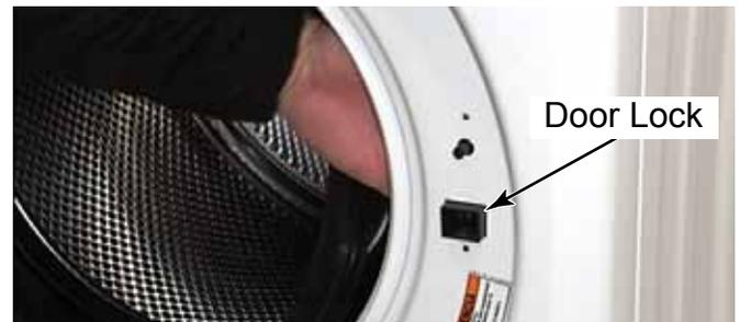
15. Reinstall the two screws, removed earlier, to mount the door lock to the front panel.
