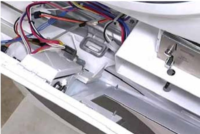
4. Place hook on bottom edge of the service switch bracket into metal hoop to hold the control panel open in the service position.
