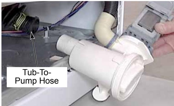
15. Pull the pump out of the washer as far as it will go.
