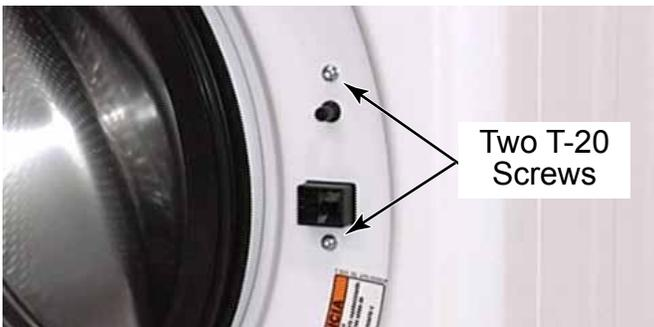
5. Remove the spring loaded retainer that holds the bellow to the washer front.
